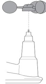
Tighten set screw with Allen wrench.
